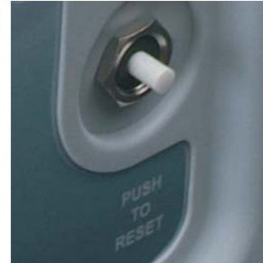
Circuit Breaker Reset
